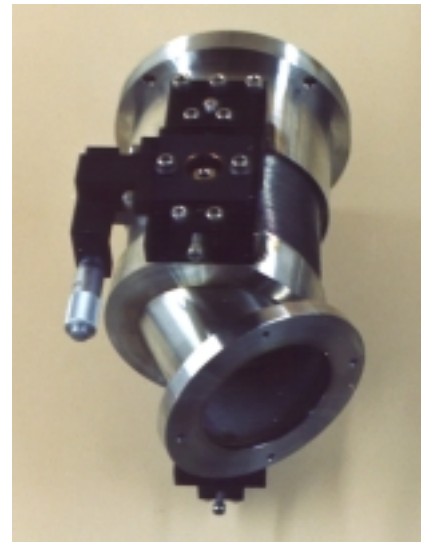
Figure 4 This ultra high vacuum compatible accessory permits to adjust a planar detector at the focal plane with respect to depth of focus and angular position.
