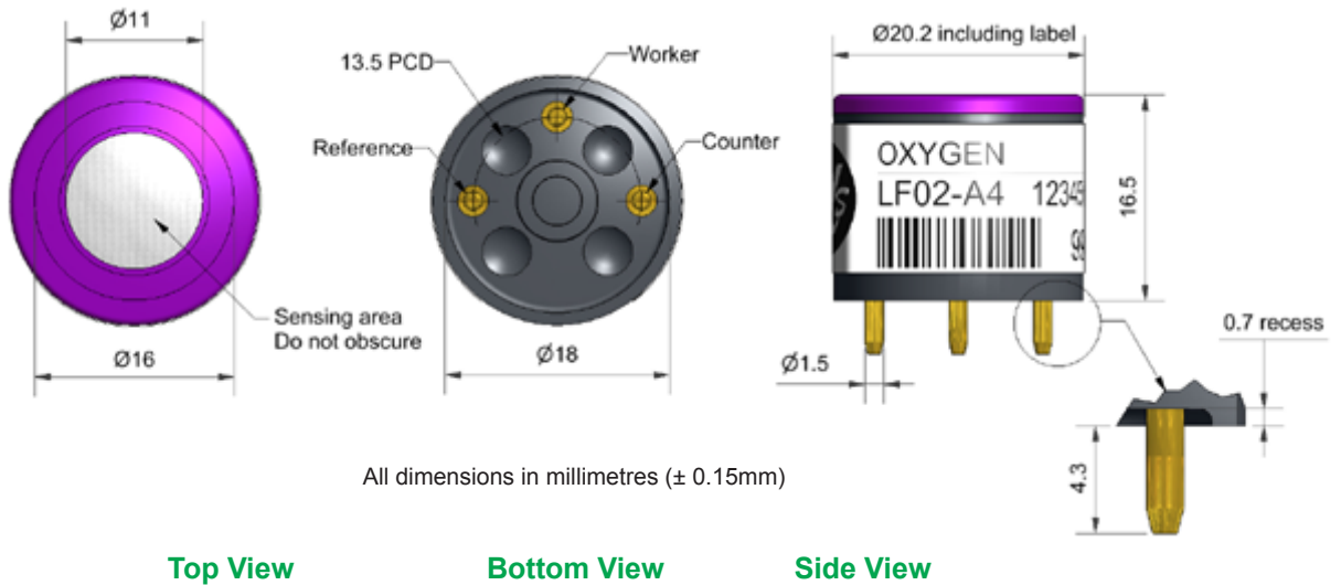
Figure 1 LFO2-A4 Schematic Diagram
